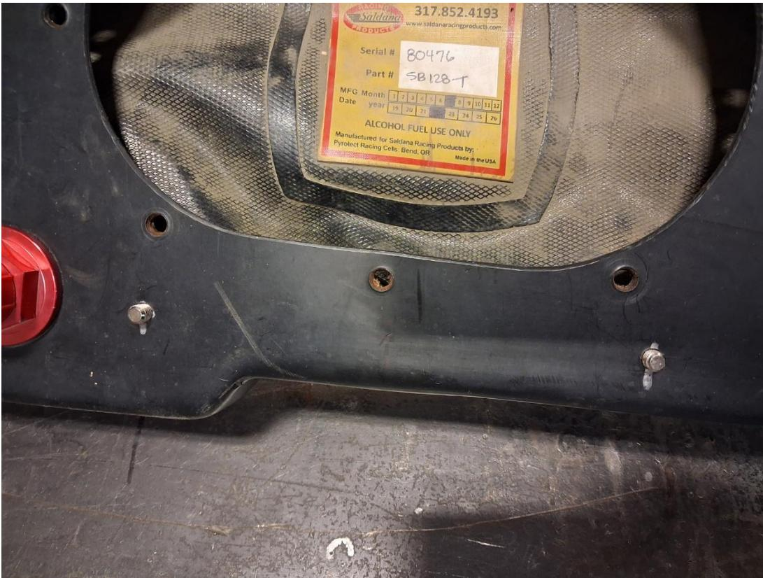
**Step 6: Finger tighten the two clevis's onto the bolts.
